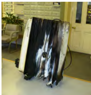
Figure 2: This portable heater had been covered and was the cause of a serious fire
