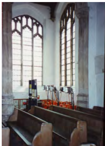
Figure 8: Gas cylinders should be stored securely and safely, not in an accessible area of the premises as in this case (5.6.13)
