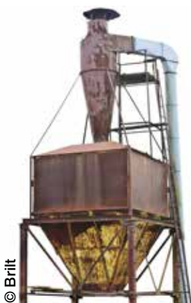
Figure 5: Dust cyclone
