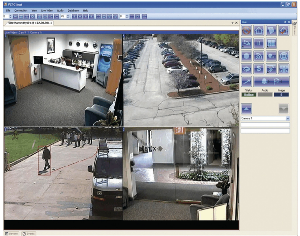
Figure 14: Example of an RVRC operator's screen: here the ADPRO VideoCentral Platinum® platform with VA in operation is both detecting and tracing the route of the target
