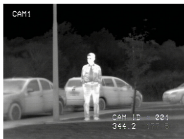
Figure 5: The observer might 'recognise' the individual but, for practical purposes, thermal images are unlikely to meet an acceptable standard for 'identification'
