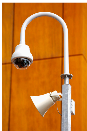
Figure 13: Camera with audio challenge facility
