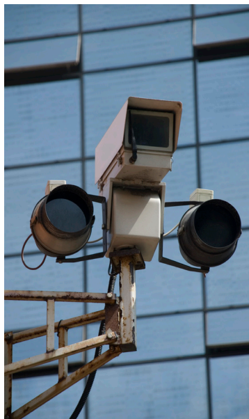
Figure 3: Traditional PTZ camera with on-board IR lighting
