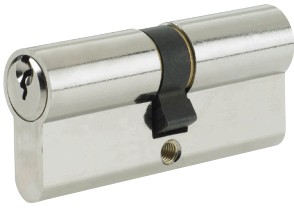
Figure 3: Typical Euro profile cylinder. Note thinness of the metal casing around the side securing screw position, ie below the moving mid-point lock cam
