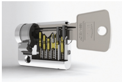
Cutaway image of a Euro profile cylinder, showing how a key engages with the (six in this case) internal cylinder pins
