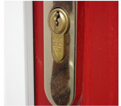
This cylinder (Note it's 'Kitemarked' but not TS 007 Star rated) sits correctly flush with the door furniture
