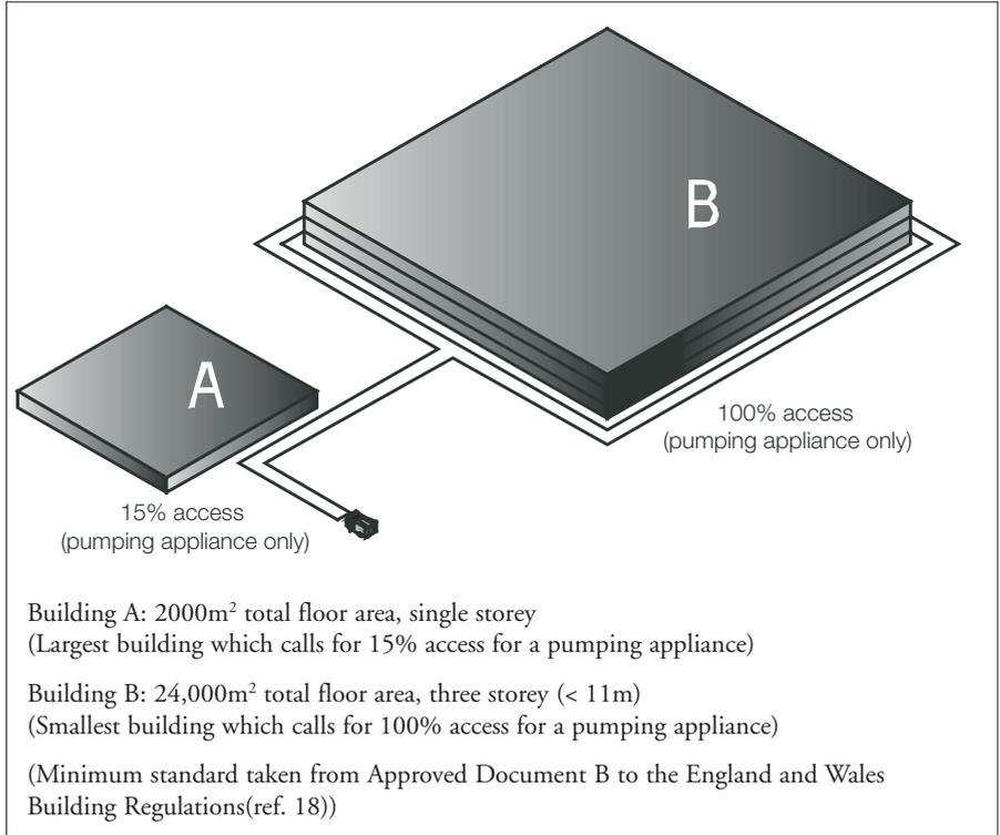
Figure 6.1: Illustration of life safety requirements for fire and rescue service vehicle access to high-risk buildings and buildings not fitted with fire mains or sprinklers
