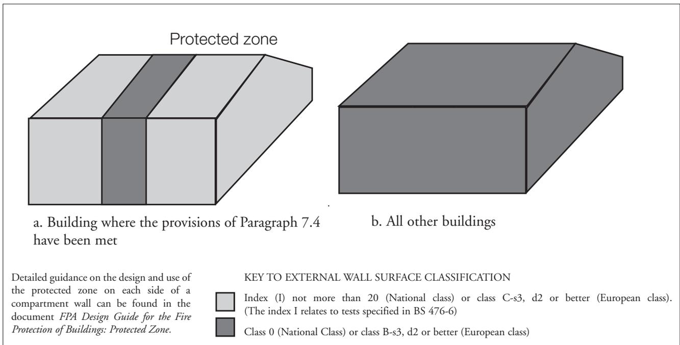
**Figure 4.1 Provisions for external surfaces of walls**
