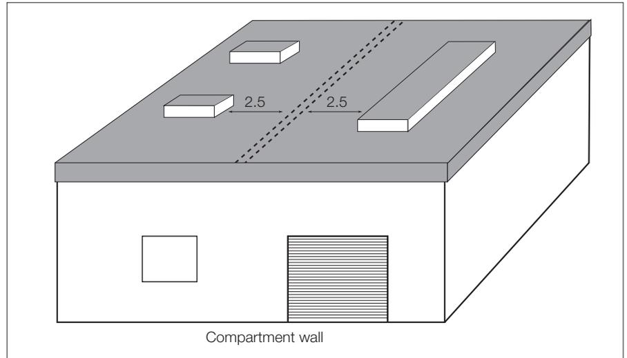
Figure 4.4: Location of roof lights from compartment wall
