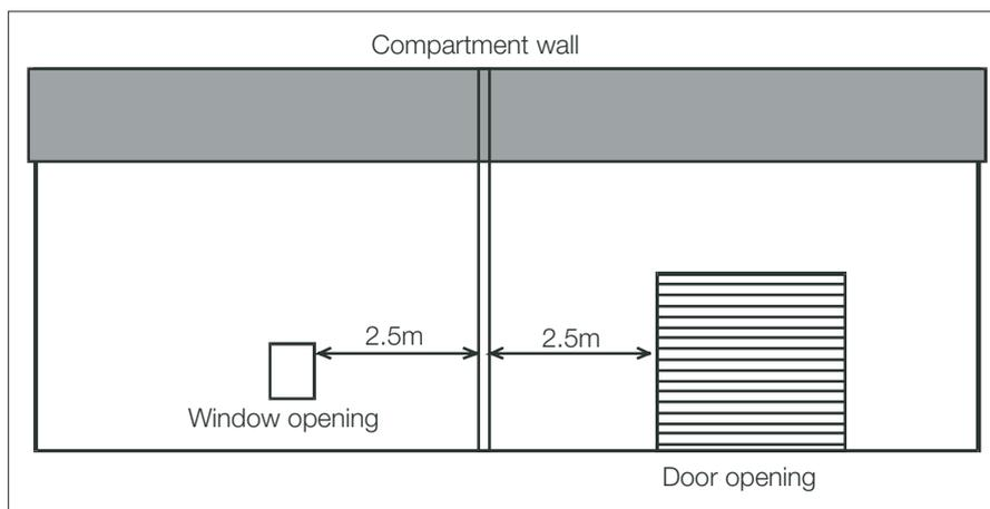
Figure 4.2: Minimum distance between unprotected openings and compartment wall
